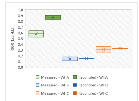
Figure 2 - Gas to oil ratio before and after reconciliation: measured/reconciled values and related uncertainties
