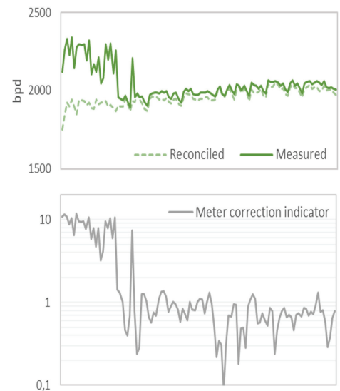
Figure 1 - Comparison between measured and reconciled flow rate and related meter quality index
